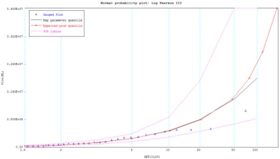
Figure A4.2: Comparison of flood frequency plots derived from peak discharges and flood volumes at Yarraman
