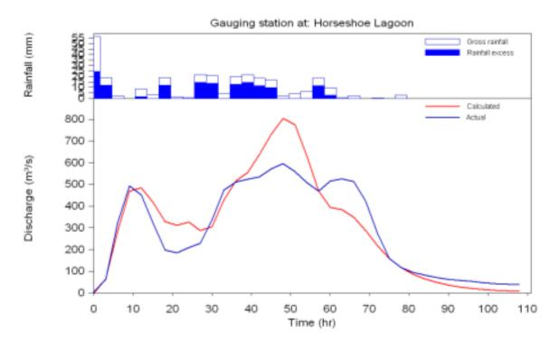
Figure A6.2: Hyetograph and calibrated hydrograph for the February 2012 flood event November 2011
