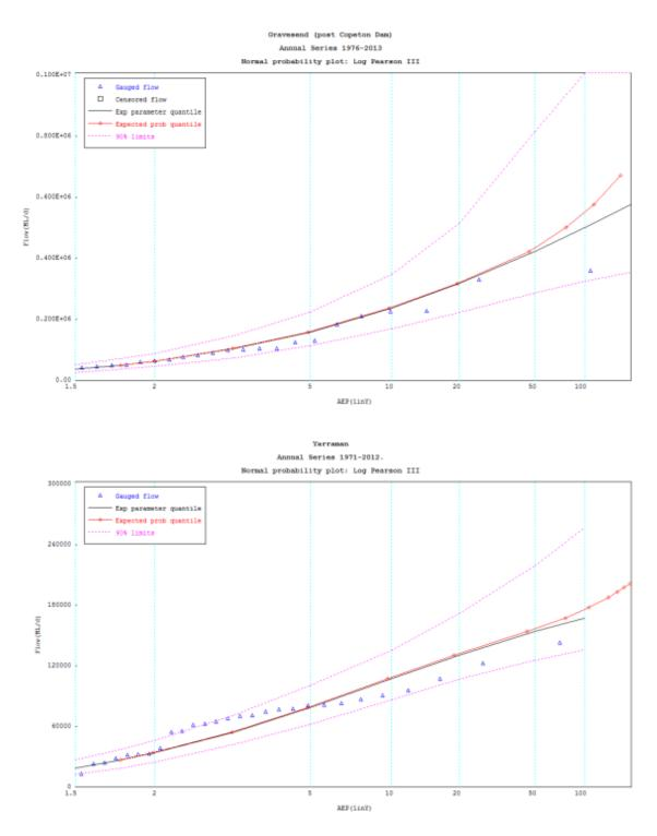
Figure A4.1: Flood frequency curves for Gravesend (post Copeton Dam) and Yarraman
