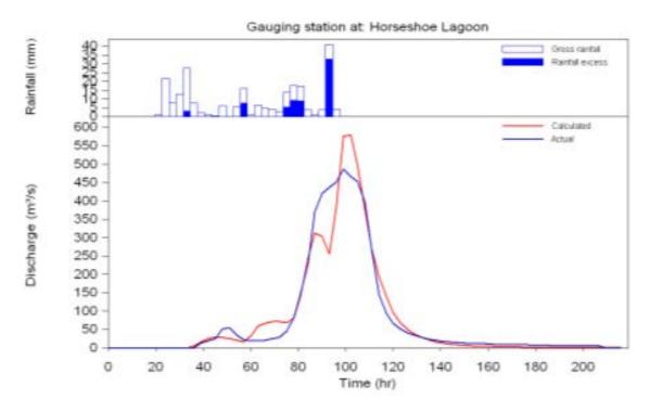
Figure A6.3: Hyetograph and calibrated hydrograph for the November 2011 flood event
