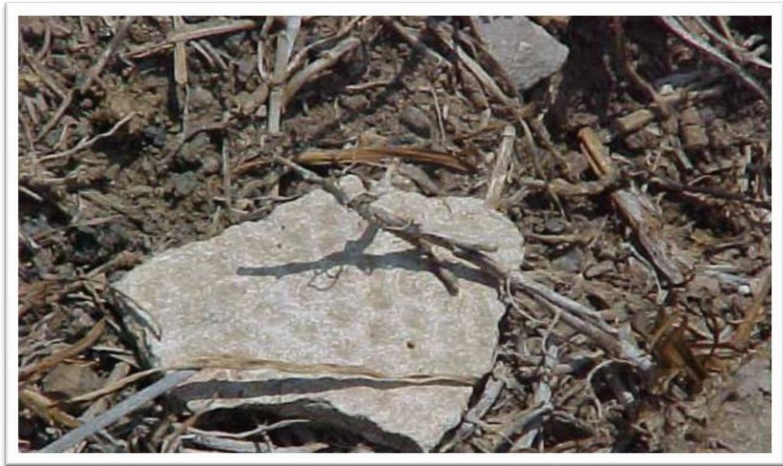
Figure 10 - Example of non-friable (bonded) asbestos fibrous cement fragment, considered to be in fair condition.
