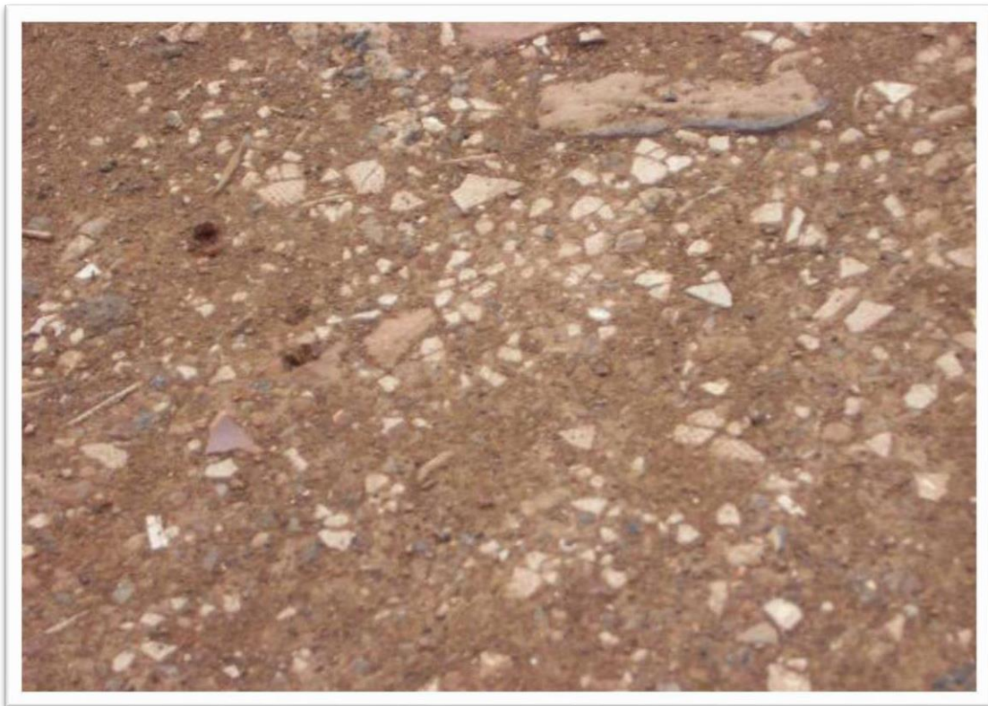
Figure 11 - Example of widespread asbestos impacted surface soils
