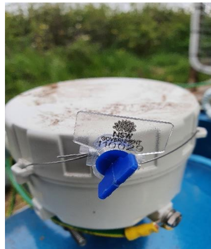
Figure 11. DQP seals on the flange bolt and the flow meter termination enclosure
