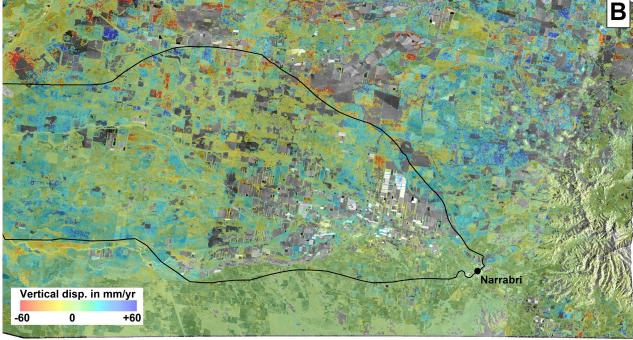
Figure 8 Ground level change along (A) the ground-satellite angle, referred to as Line Of Sight (LOS), and (B) projected along a vertical axis. Note that InSAR directly measures (A). (B) is inferred by considering the horizontal component of motion as being negligible (A). Due to the SAR acquisition geometry, velocity values in the horizontal direction are slightly higher than values measured along the LOS angle (≈35 degree). The groundwater model boundary is shown as black line.
