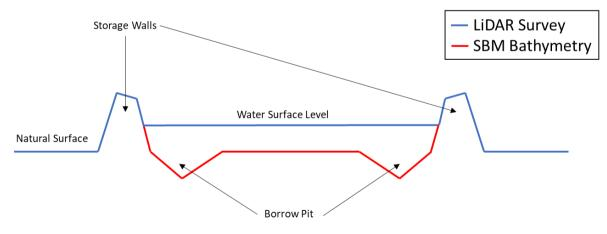
Figure 1 Conceptual representation of an OFS and the SBM bathymetry
