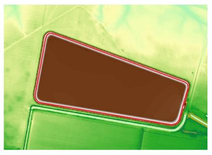
Figure 3 Example storage outline (red line) when compared to the DEM (background colours)
