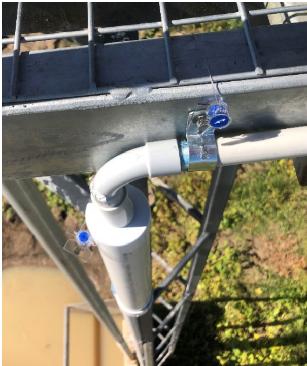
Figure 3 Image shows a tamper evident seal fixed to a pressure sensor on a catwalk.
