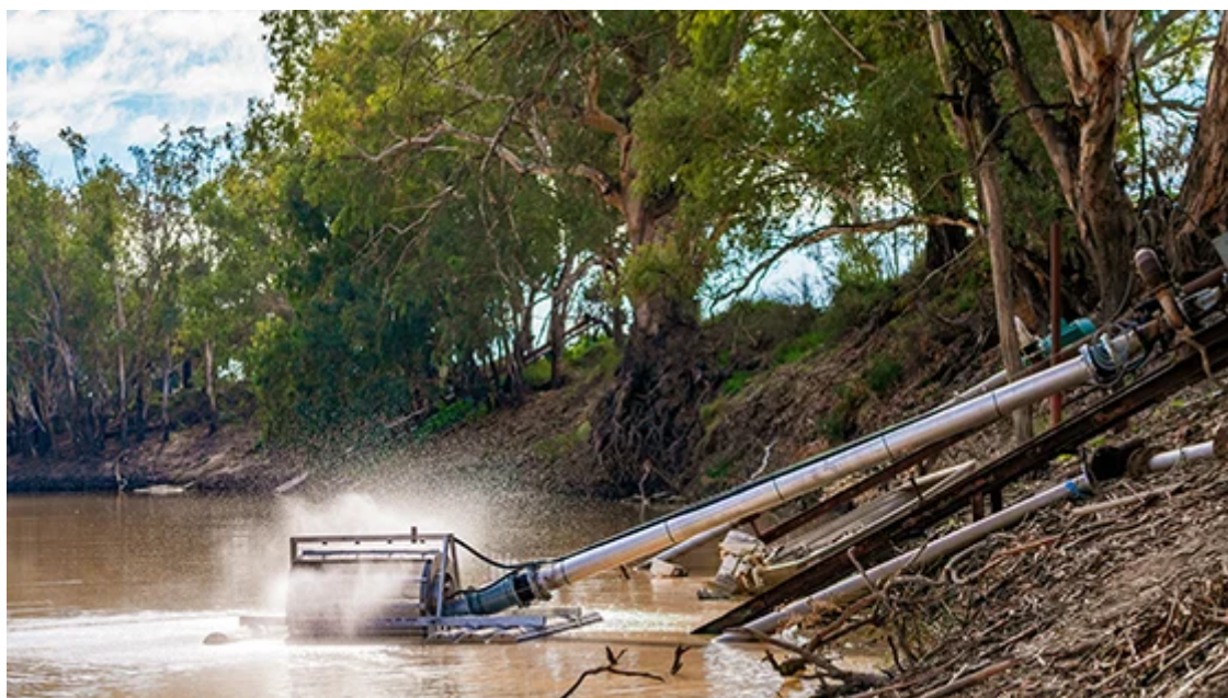
8-inch Riverscreen floating diversion screen operating at Porker Citrus on the Darling. Photo credit: David Sickerdick
