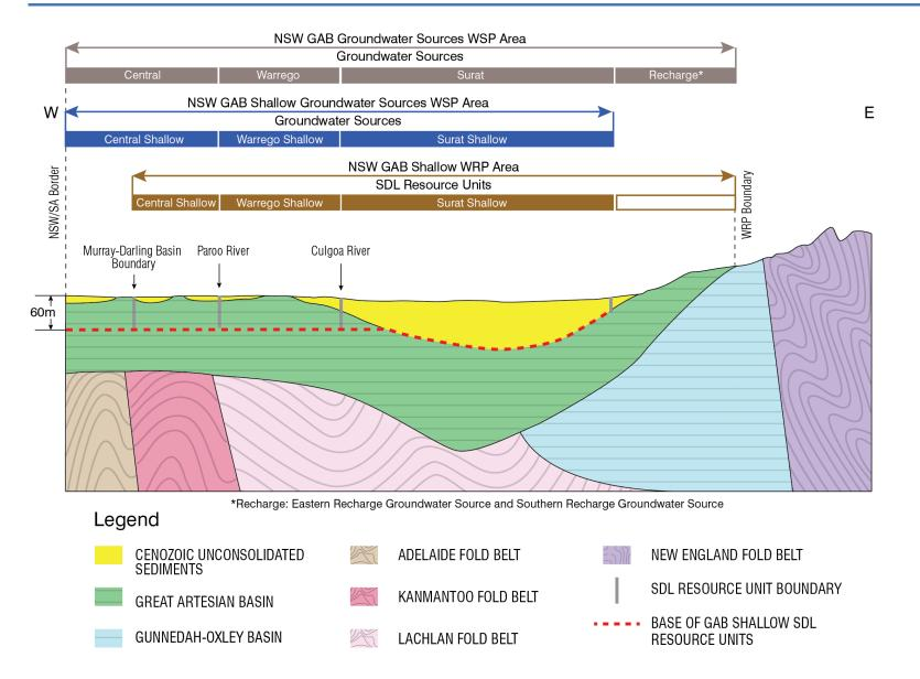
Figure 2 Schematic cross section of the SDL resource units in the NSW Great Artesian Basin Shallow WRP area and their relationship to the NSW water sharing plans and their groundwater sources
