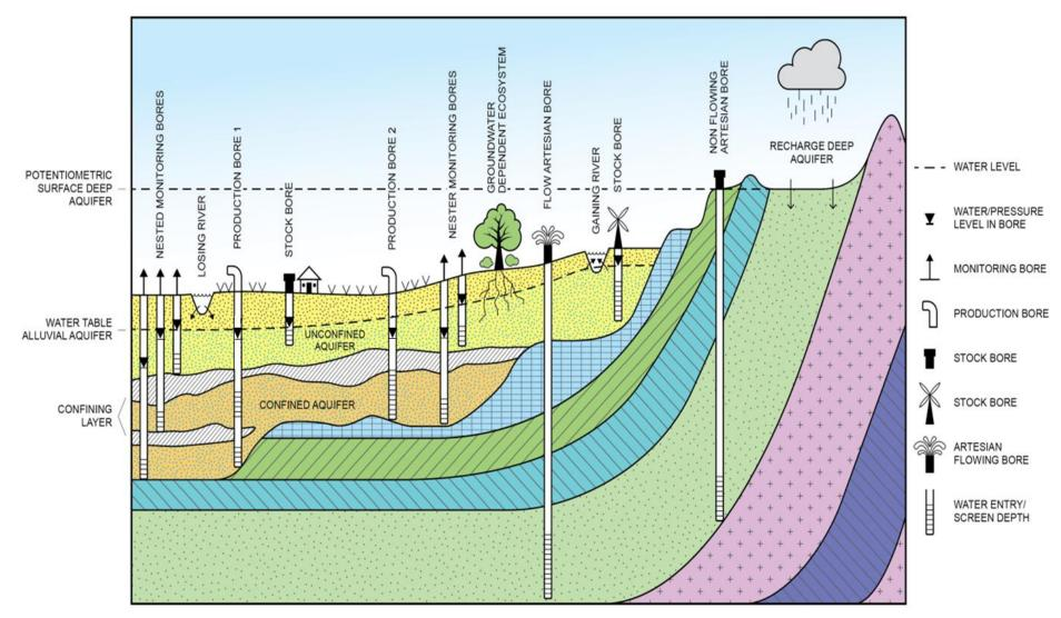
Figure 19 Schematic diagram of different types of aquifers
